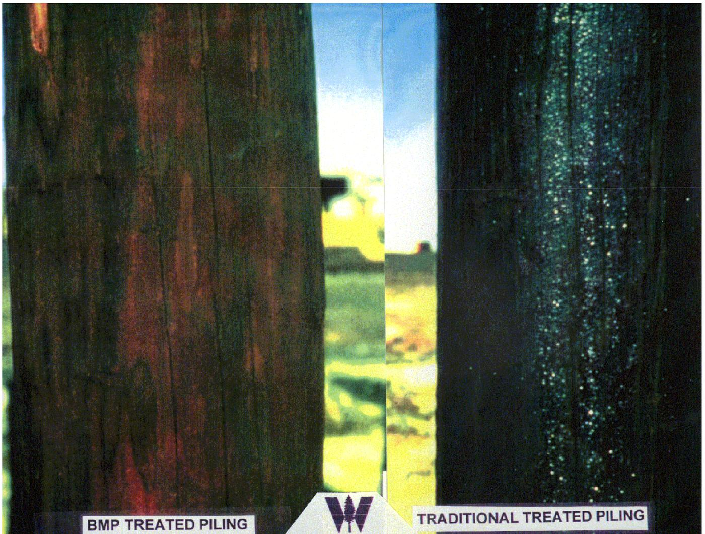
**Fig. 2.** A new pile treated with creosote to BMP standards, prior to weathering, compared to a pile treated to traditional standards. Note the obvious residual surface creosote on the pile receiving the traditional treatment. (Photo courtesy of R. D. Hayward.)
