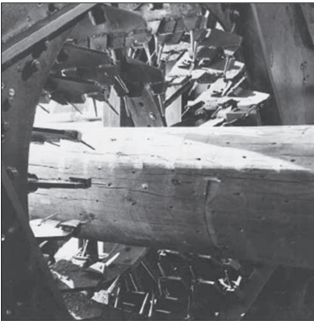
Figure 15-4. Deep incising permits better penetration of preservative.
