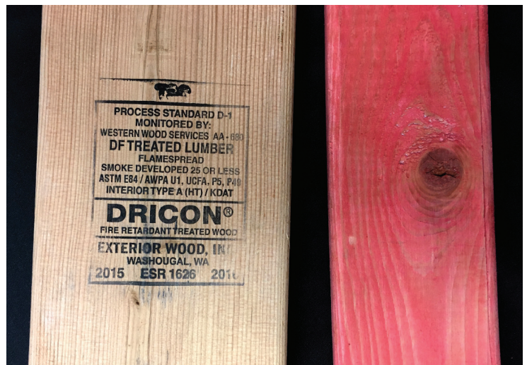
Color should not be used as the only indicator for fire retardant-treated wood. The best identifier is the code-required quality mark, which assures the wood has been infused with the approved fire protection.
