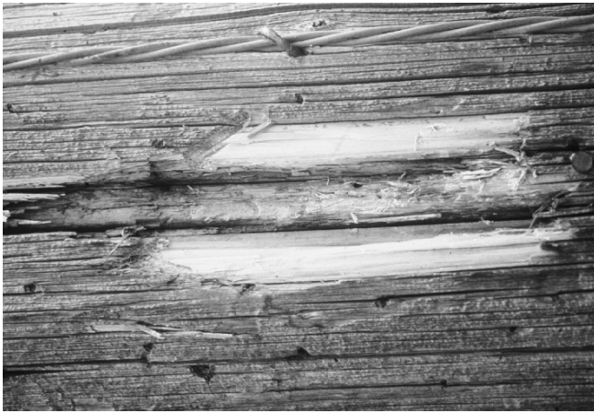
Figure 1.3 Example of weathering on wood showing the gray color and the lighter wood beneath.
