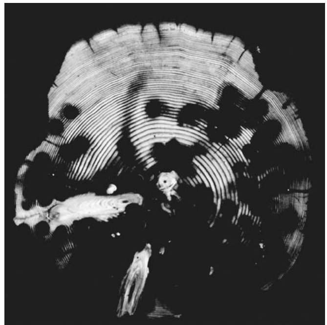
Figure 1.7 Cross section of wood damaged by shipworms showing extensive calcium lined tunnels in the interior.
