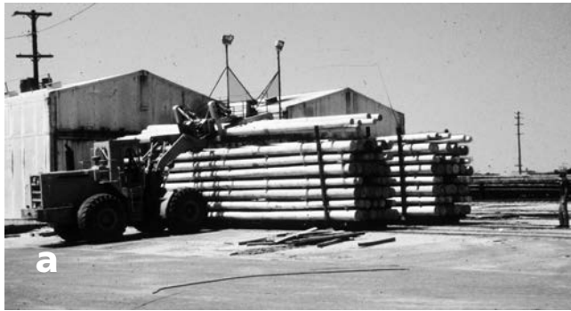
Figure 2.8 Stacked poles (a) and lumber (b) being prepared for a batch kiln.
