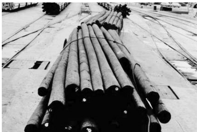
Figure 2.14 Pole stock subjected to a final steam/vacuum cycle.
