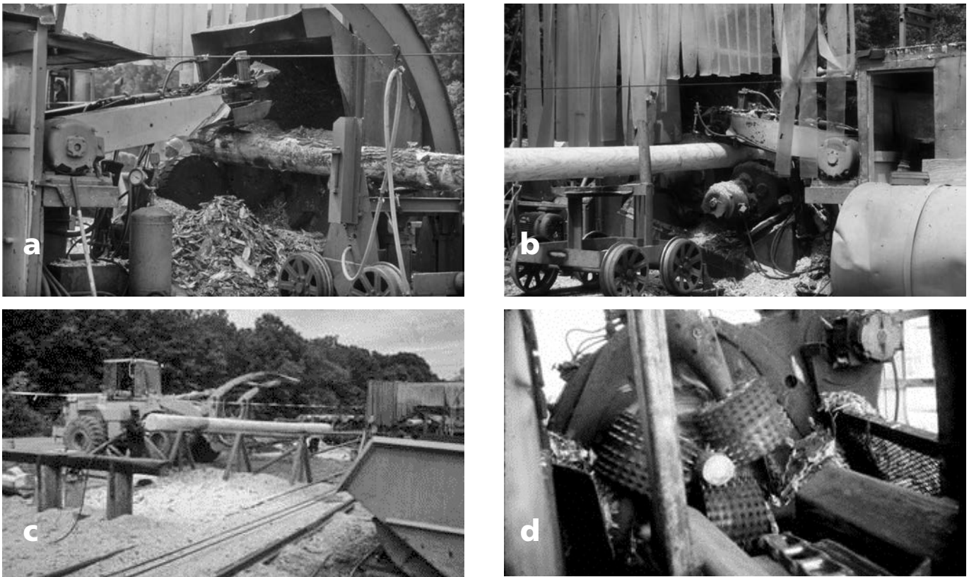
Figure 2.2 Typical pole peeler (a, b, c) and Cambio ring debarker (d) used in de-barking operations.
