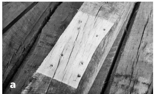
Figure 2.5 Typical conventional (left) and double density (right) incising patterns for dimension lumber
