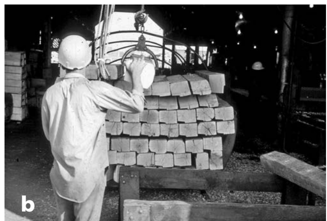
Figure 2.6 Adzed and bored tie plate area (a) and machined stock (b) will increase service life of crossties (a) and crossing plank (b).
