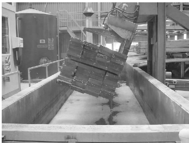
Figure 2.13 Dipping lumber bundles for diffusion treatment.
