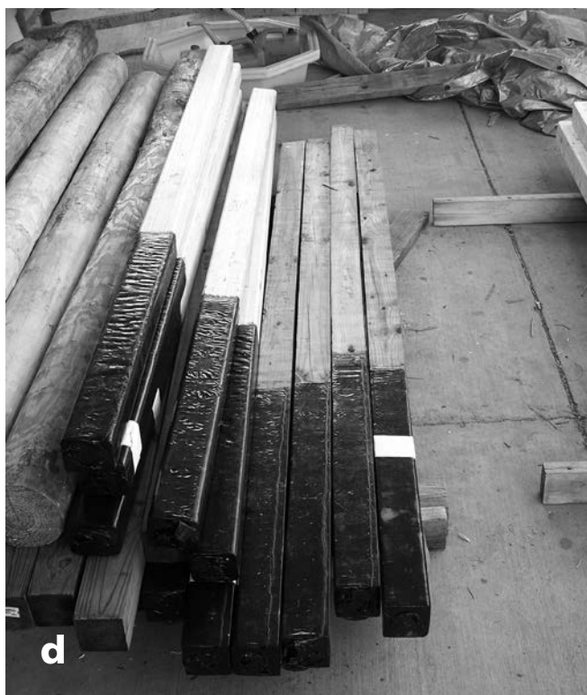
Figure 2.15 Typical barrier wraps for round and rectangular sections. From (a) http://www.postprotector.com ; (b) http://www.pplfieldliners.com/users.htm ; (c) http://www.pplfieldliners.com/users.htm ; (d) Barnes et al. (2009).
