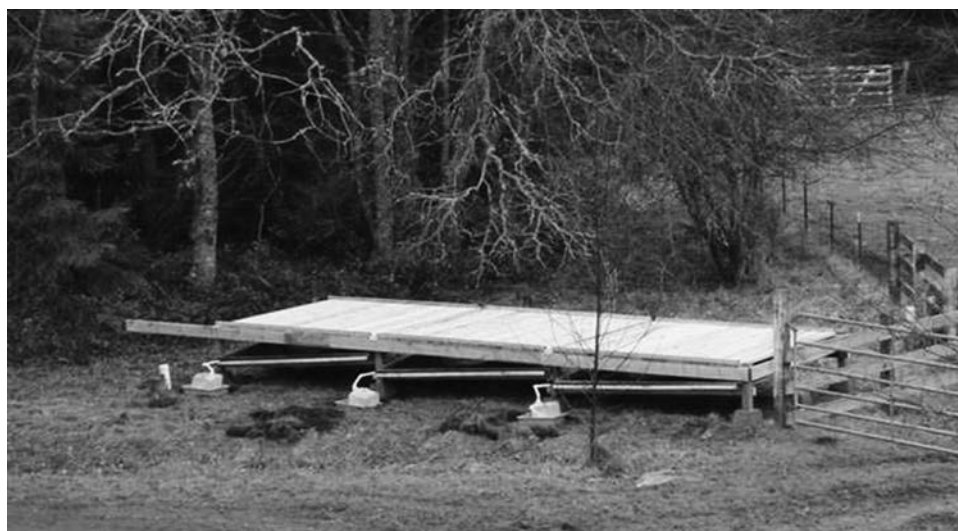
Figure 5.5 Experimental decks with installed Cubitainers™ ready to collect the first 1.5 cm of rainwater runoff. Two of the decks are covered with southern pine treated to a mean retention of 0.24 kg/m 3 Wolman AG™ preservative.
