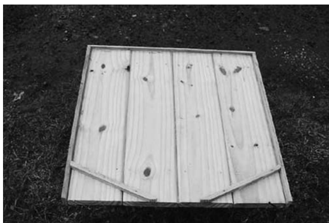
Figure 5.6 Wolman AG™ preserved southern pine deck used to collect the first flush of rainwater for a replicate chronic freshwater algae bioassay in March 2008.
