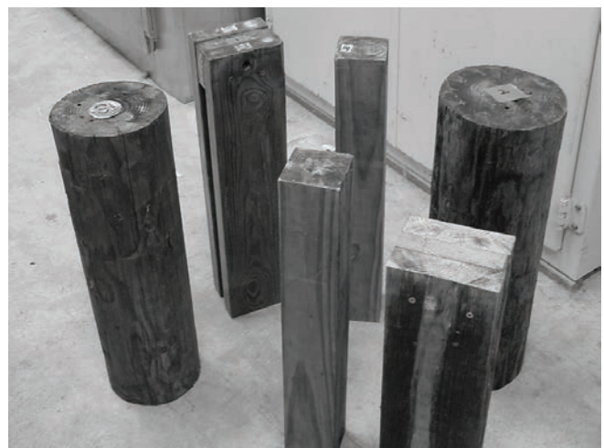
Figure 7.2 Commodity size samples used to evaluate preservative loss rates.
