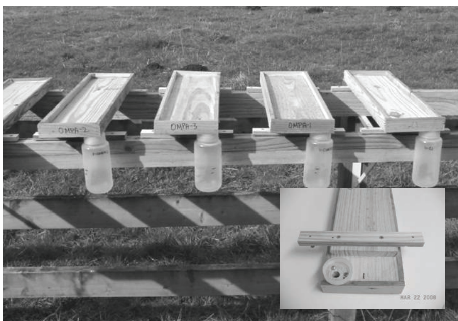
Figure 7.29 Example of pressure-treated decking samples evaluated during rainwater runoff studies.
