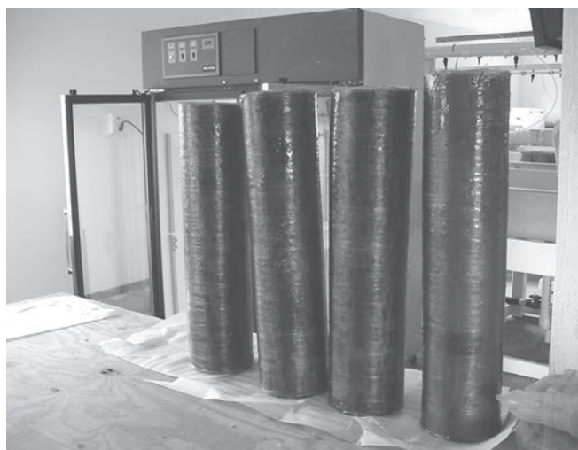
Figure 11.8 Three Strong-Seal fiberglass-wrapped CCA-treated wood piling and a similarly wrapped control.
