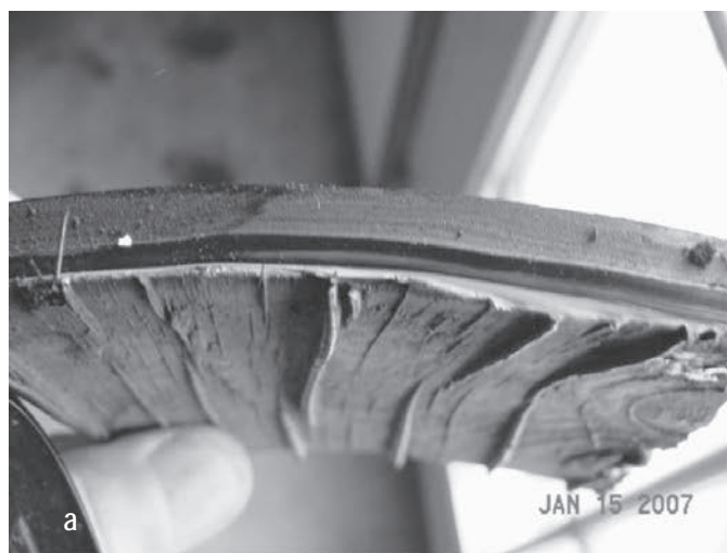
Figure 11.11 (a) Breach of the TIP HDPE piling wrap with adhered surficial layers of ACZA treated wood and (b) breach of the untreated piling with no adherence of the underlying wood fibers.
