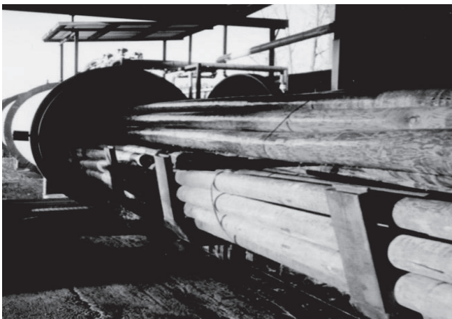
Figure 11.3 Fixation cylinder and wash down system used to satisfy BMP requirements for CCA-C treated piling at Wood Preserver's Inc.
