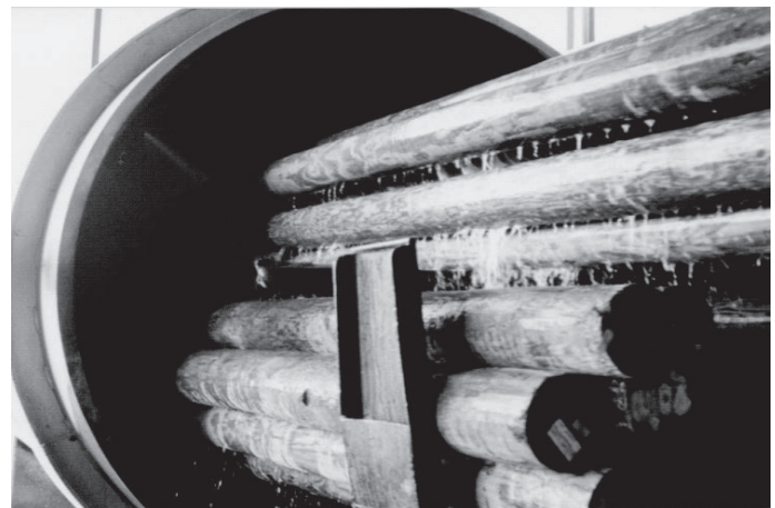
Figure 11.3 Fixation cylinder and wash down system used to satisfy BMP requirements for CCA-C treated piling at Wood Preserver's Inc.
