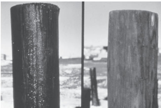
Figure 11.2 Traditional (left) and BMP creosote piling.
