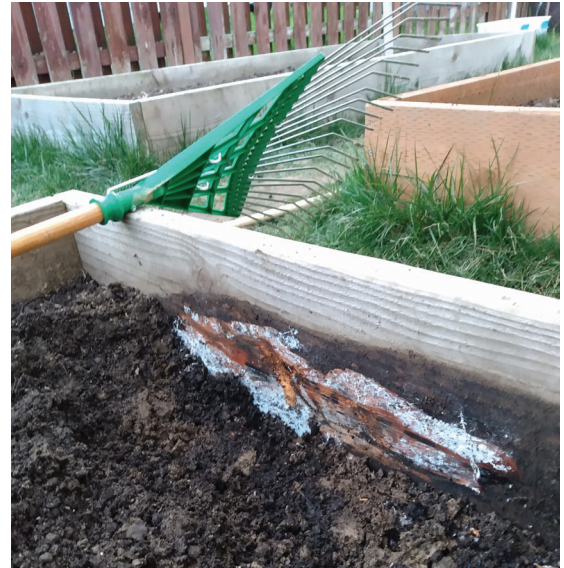
Boxes constructed from untreated wood showed signs of decay after only one year of use. The preserved wood boxes had no evidence of deterioration when exposed to the exact same outdoor conditions.
