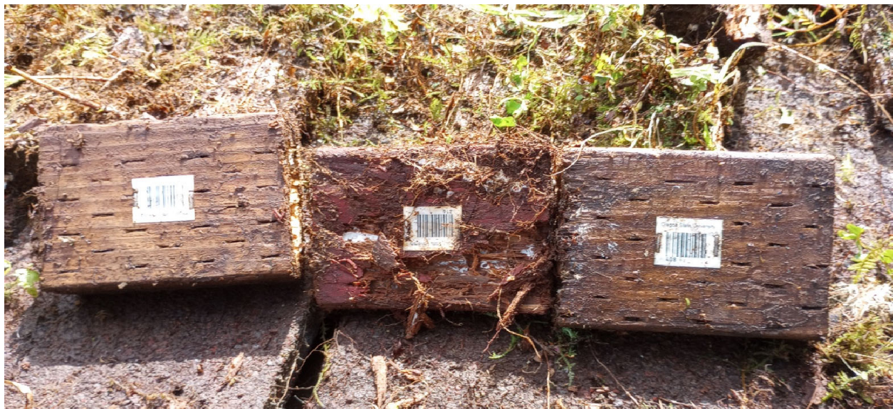
Figure 7. Examples of EcoRed Shield I (middle) and Copper Azole (left and right) ground proximity samples after 108 months of exposure. The EcoRed Shield I sample pictured was the only remaining sample at this timepoint that had not failed.
