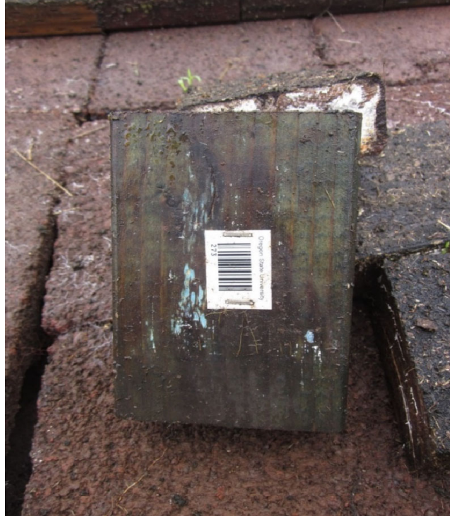
Figure 6. BluWood ground proximity sample after 24 months of exposure showing decay pockets with concentration of the original blue dye used to color the wood.
