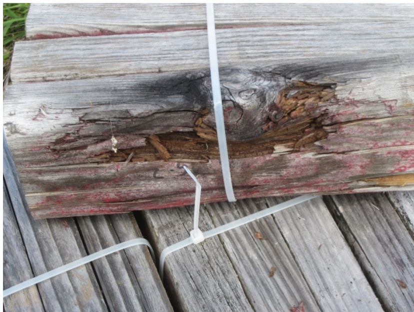
Figure 9. Example of an EcoRed Shield I sandwich with extensive decay on the outer sample after 30 months of exposure. Interestingly, this sample remained in service through 72 months despite this early decay damage.
