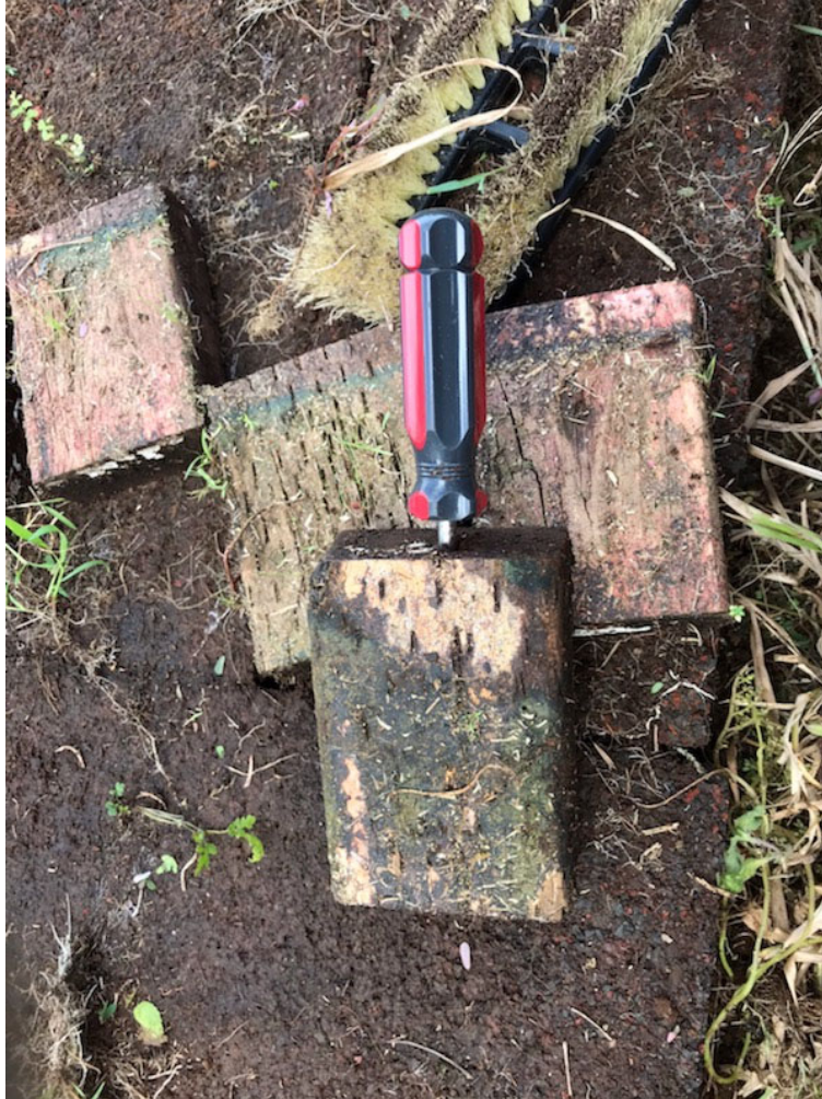
Figure 9. Example of a copper azole-treated ground proximity specimen showing a sound exterior but decay in the cut, exposed end grain. This effect was seen from 72 months onward.
