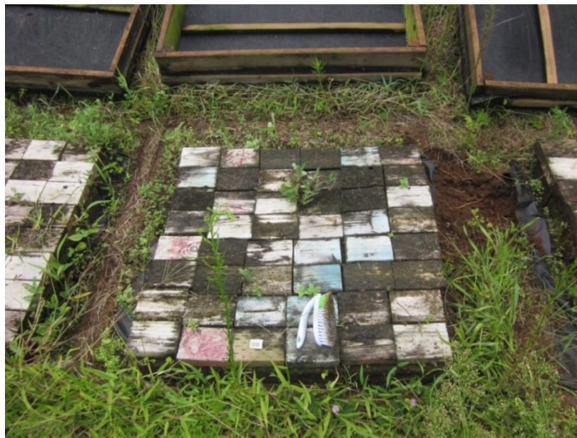
Figure 3. Example of an E18 Ground proximity decay test prior to the 18-month assessment.
