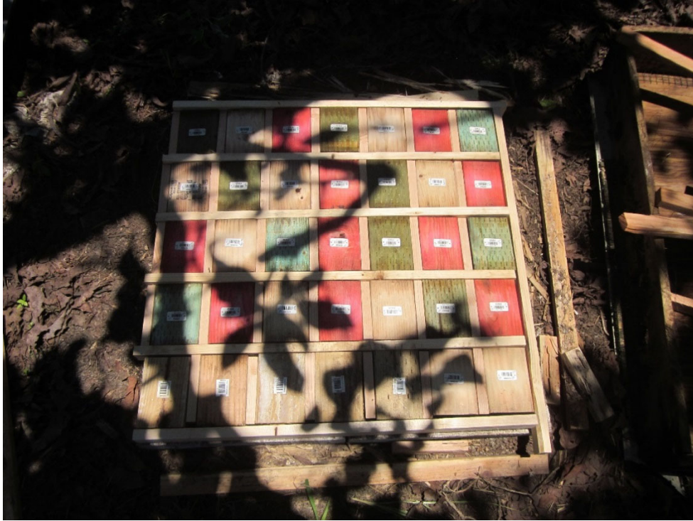
Figure 2. Example of a termite array with samples treated with EcoRed Shield II, HiBor or left untreated in the E26 Ground Proximity termite test after installation in June 2015.
