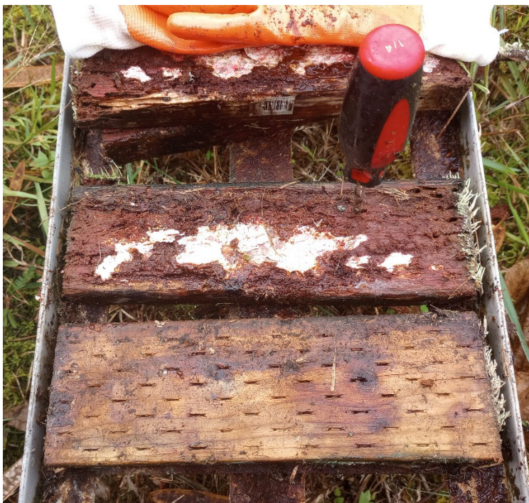
Figure 10: Example of sandwich test sample condition after 108 months of exposure. An EcoRed I sample is completely degraded and can be penetrated with a screwdriver, whereas a copper azole-treated sample at the bottom of the photo is in much better condition.
